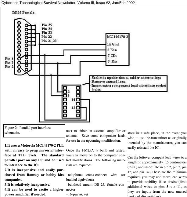
Building the kit is straight forward. The only modification I would make is to Remove U2, the PIC microcontroller and
