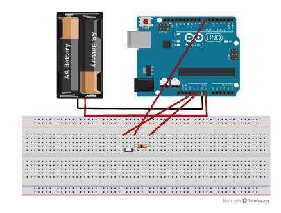
What we have here is a diagram of a simple sensor switch hook-up with an Arduino. You can program it to detect a change in the switch's state, so this works with both Normally Open (NO) and Normally closed (NC) switches.
