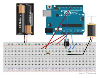
The schematic is the same as the previous one, but now we have a solenoid being driven by a MOSFET when activated by the Arduino. Again, this is straight out of Banzi's book.
