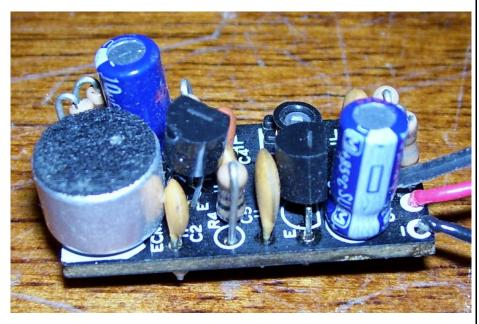
This picture is an assembled Radio Shack 28-4030 FM Wireless Microphone Kit. The kit was reviewed Issue #10 of **The Cyberpunk Technical Journal**, and this particular model is a typical design. It operates in the low end of the FM Broadcast band, around 88-92 MHz., and has an advertised range of about 50 feet when run off a 1.5 Volt battery.
