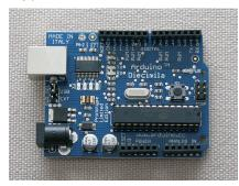
It's programmed via a USB connection, can run on batteries, and has a number of digital and analog I/O lines that let you hook up any number of sensors or other devices. Hopefully by now you can think of a few ideas for this.
