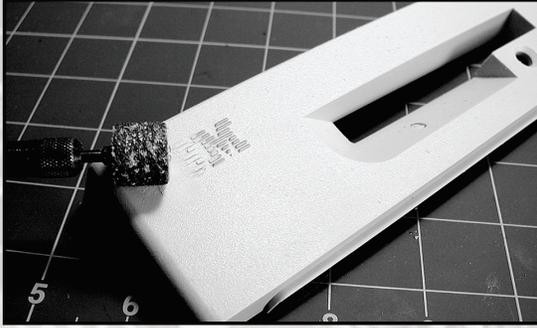
Fig. 4: Grinding off the IBM logo.
