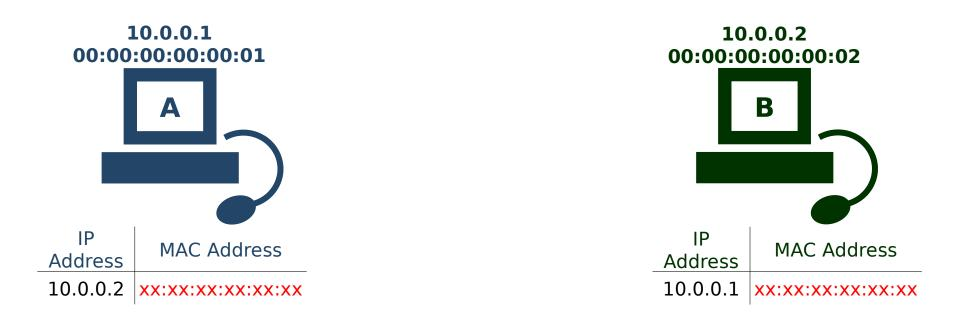
Even when X leaves the network, A & B still have each other's IP address assigned to the MAC of X. Since X is no longer on the network, the frames go nowhere.
