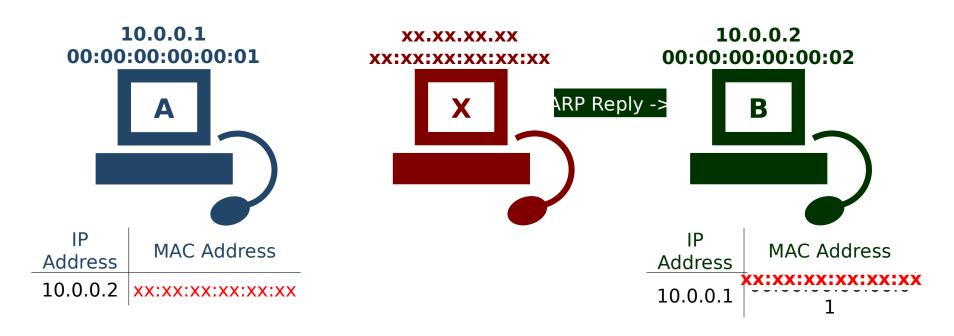
Computer X then sends a spoofed ARP reply to computer B. This reply replaces the IP address of A with the MAC of X.
