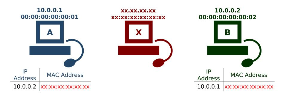
Computer X needs to do one more thing to prevent disrupting the communication Between A and B. It must forward the packets A sends to B on, and visa versa.
