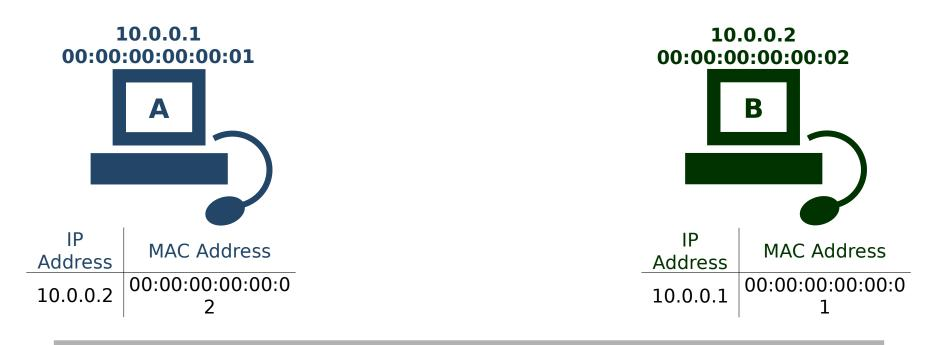
Computer A & B are communicating on a switched network. (For illustration purposes, switch left out of picture.)
