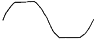
This is a sine wave with its peaks flattened (or cut off). It causes distortion, harshness, and trouble. A telephone earpiece has a dual diode connected across the terminals in newer units, and if the signal level is too great the diodes absorb the peaks of the sine wave, thus causing the waveform to distort like this. Remove the diode before using.
