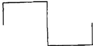
A square wave, generated by an on-off type of device such as a multivibrator, has a lot of harmonics, sounds harsh and is not as effective as a sine wave, though often easier to make.
