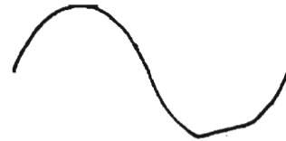
A Twin T oscillator slightly distorted, because it is tuned 5% higher than its initial frequency of oscillation. Its stability is excellent. It's dynamite for boxing.
