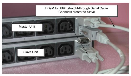
The **CONTROL OUT** Port is a DB9M Connector used to cascade **PCU8** boxes.
