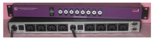
The easy to use, easy to configure **PCU8** provides the means to control all devices with simple commands to turn Power Off / On to reboot any one port, multiple ports, port groups or all devices. Power restarts can be sequenced using programmed time delays to minimize surge or allow drive spin-up time. Front panel controls and indicators are also provided to show the status of each port.
