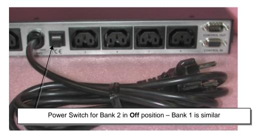
The Power Switch is off when the white band is showing (as above). When the circuit breaker has tripped, the white band will show; the overload condition should be corrected before restoring the circuit by pressing the switch in to reset it.
