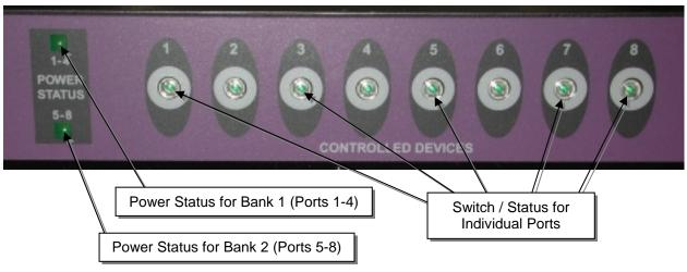
The front buttons can be disabled to prevent local control of switched devices; the indicator lamps will always operate. Each indicator is a green LED for an 'on' condition.
