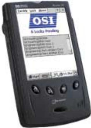
The Windows CE or PocketPC devices are **required** for programming any of the **OMNILOCK** OM2000 or OP2000 locks. Additionally, these devices may be used to program the newer generation of OM100, OM300, or OM500 Series locks. One CE Device will work with any number of locks.
