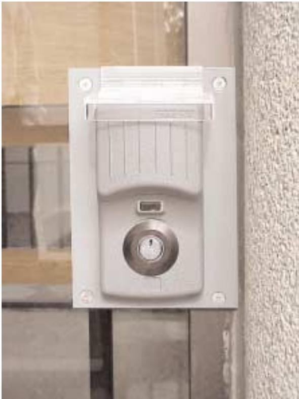
The versatile Wall Mount System may be used to control electric strikes, magnetic locks, electrified exit devices, elevator control boxes or any electric circuit of 12-24 VDC/RMS voltage, 5 amperes (shown with upper door of SP2 weatherized cover installed- see page 32 for details)
