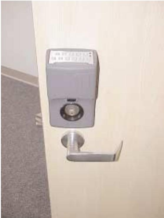
Built on Grade1 Falcon or Schlage Mortise or Mortise-with-Deadbolt. Standard or IC Core cylinders available, Accepts 1<sup>3</sup>/<sub>8</sub> inch to 1<sup>3</sup>/<sub>4</sub> inch mortise cylinder. The Mortise collar p/n 11445-001 is required for 1<sup>3</sup>/<sub>8</sub> cylinders.
