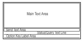
The Entering Text screen shows the areas where you can enter text. Unlike typical keyboard text entry, with the MX240a unit, you enter text via thumb typing.
