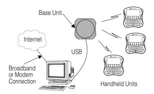
Note: One base is capable of operating with up to seven handhelds simultaneously.
