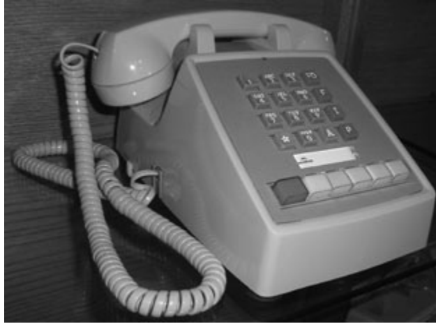
A 16-button AUTOVON telephone, whose red-colored fourth column of precedence buttons made the military telephone network a sensitive and seemingly irresistible target for certain phone phreaks. Photo courtesy Wayne Merit, JKL Museum of Telephony
