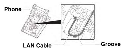
3 Lead the LAN cable out through the groove on the tilt leg, as shown in the figure below.
