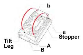
While pushing the two hooks, slide the tilt leg downward. Remove the tilt leg from the terminal.
