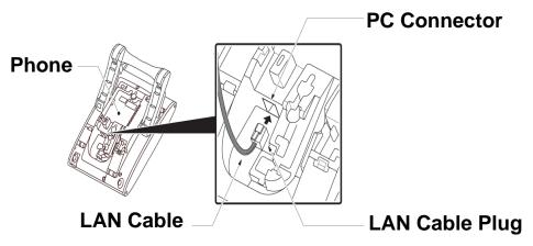
2 Thread the LAN cable through the groove on the back of the phone.
