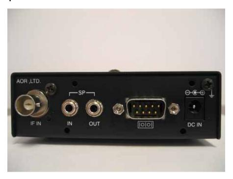
The rear of the ARD25 has one (1) DB-9 connector for connection to a PC, one (1) BNC connector for IF input, one (1) DC power connector, one (1) speaker input, and one (1) speaker output.
