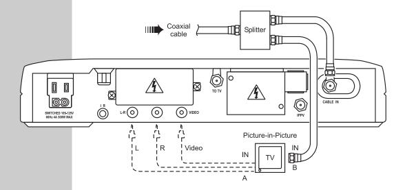
Use this diagram to record how the CFT2200 is connected in your TV system.
