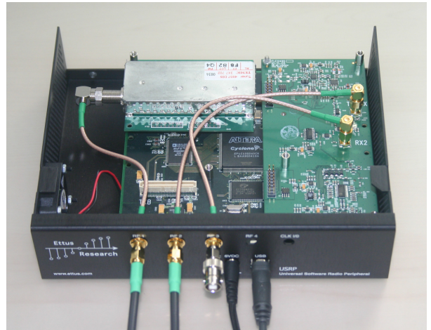
Figure 2: The USRP Software-Defined Radio with 80–870MHz VHF/UHF receiver (top left) and 400–500MHz UHF transceiver (right) daughter boards.
